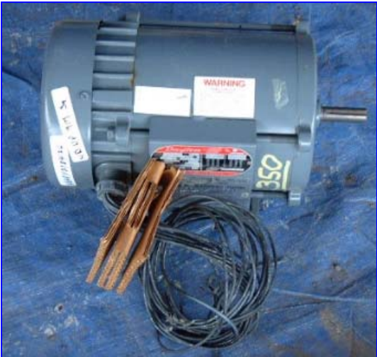
Dayton Motor, 1,725/1,425 rpm, 3.4hp, 230/460 volt, 2.4/1.2 amps, 60/50 hz, 3 phase, G56 Frame.
