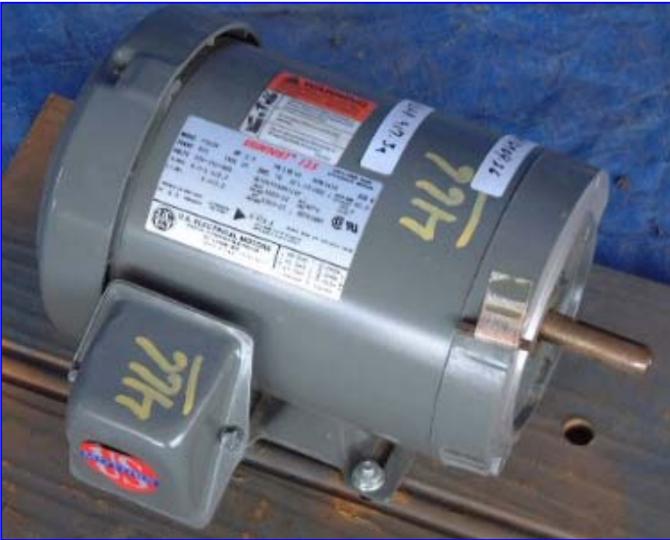
US Electrical Motors, 2 hp, 3,450 rpm, 208-230/460 volt, 6.0-5.3/2.7 amps, 60 hz, 3 phase, 56C frame.
