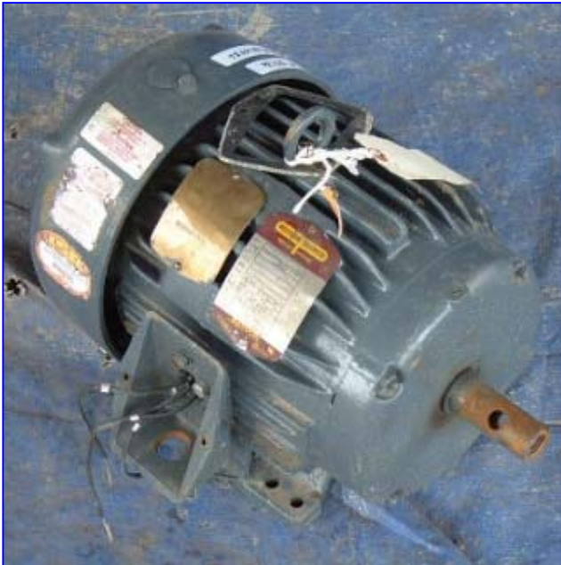
Baldor Motor, 3 hp, 1,750 rpm, 460 volt, 4.1 amps, 60 hz, 3 phase, 182 TZ.
