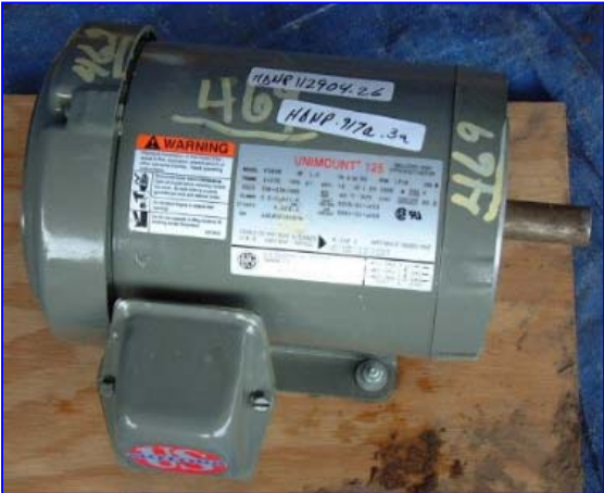
US Electrical Motors, 1 hp, 1,750 rpm, 208-230/460 volt, 36-3.6/1.8 amps, 60 hz, 3 phase, 143 TC frame.
