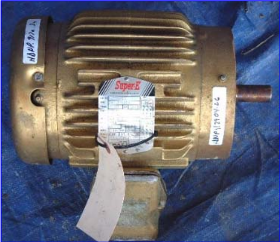
Baldor Motor, 1 hp, 1,750 rpm, 230/460 volt, 4.2/2.1 amps, 60 hz, 3 phase, 145 TC frame.
