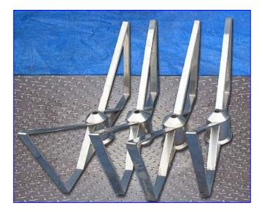
(4) Stainless Steel mixing paddles. Propeller dimensions: 44 in. L x 17 in. H. Shaft diameter: 1-1/4 in. Overall dimension: 44 in L x 17 in. H.
