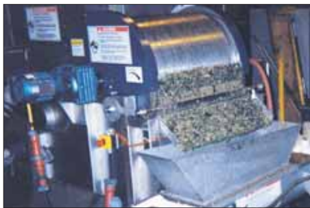
The Rotostrainer screens discrete solids, scum and oily materials without blinding
