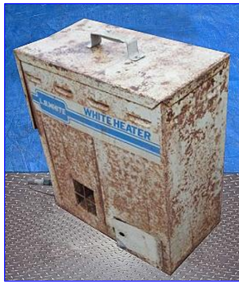
(1) L.B. White Direct Fired Circulating Construction Heaters. Model: 348G. S/N's: 18605. Capacity (input): 65,000 Btuh. Natural gas. Airflow: 250 cfm. Gas supply (max/min): 10.5/7 in. W.C. Burner manifold pressure: 3.4 in. W.C. Power supply: 115 VAC, 3 amps, 60 Hz, single phase. Overall dimensions: 21-1/2 in. L x 11 in. W x 24 in. H.
