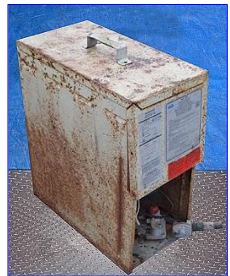
(1) L.B. White Direct Fired Circulating Construction Heaters. Model: 348G. S/N's: 18605. Capacity (input): 65,000 Btuh. Natural gas. Airflow: 250 cfm. Gas supply (max/min): 10.5/7 in. W.C. Burner manifold pressure: 3.4 in. W.C. Power supply: 115 VAC, 3 amps, 60 Hz, single phase. Overall dimensions: 21-1/2 in. L x 11 in. W x 24 in. H.
