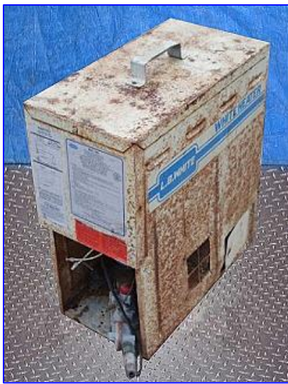
(1) L.B. White Direct Fired Circulating Construction Heaters. Model: 348G. S/N's: 18605. Capacity (input): 65,000 Btuh. Natural gas. Airflow: 250 cfm. Gas supply (max/min): 10.5/7 in. W.C. Burner manifold pressure: 3.4 in. W.C. Power supply: 115 VAC, 3 amps, 60 Hz, single phase. Overall dimensions: 21-1/2 in. L x 11 in. W x 24 in. H.
