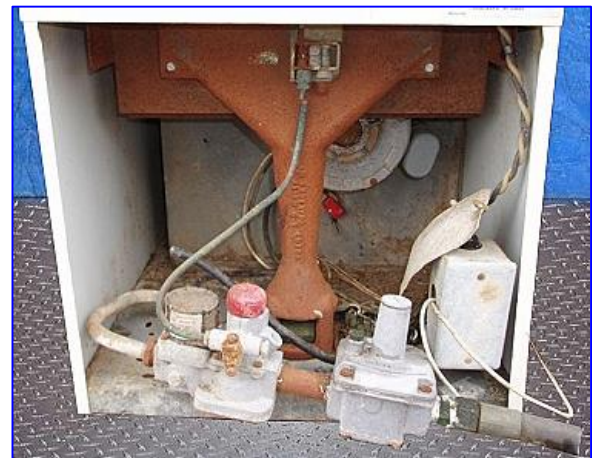
(1) L.B. White Direct Fired Circulating Construction Heaters. Model: 348G. S/N's: 18605. Capacity (input): 65,000 Btuh. Natural gas. Airflow: 250 cfm. Gas supply (max/min): 10.5/7 in. W.C. Burner manifold pressure: 3.4 in. W.C. Power supply: 115 VAC, 3 amps, 60 Hz, single phase. Overall dimensions: 21-1/2 in. L x 11 in. W x 24 in. H.
