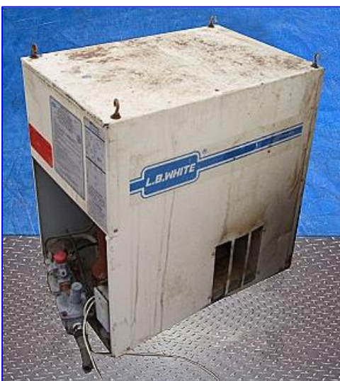
(3) L.B. White Direct Fired Circulating Construction Heaters. Model: 379G-1. S/N's: 19044. Capacity (input): 115,000 Btuh. Natural gas. Airflow: 480 cfm. Gas supply (max/min): 14/5.5 in. W.C. Burner manifold pressure: 4.5 in. W.C. Power supply: 115 VAC, 3 amps, 60 Hz, single phase. Overall dimensions: 23 in. L x 16 in. W x 24 in. H.
