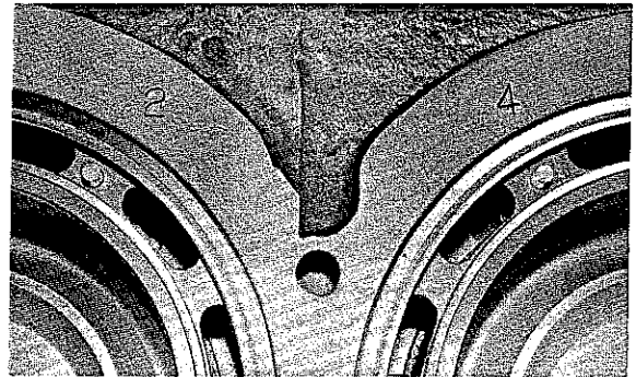
Fig. 58 Cylinder number mark (case side)
