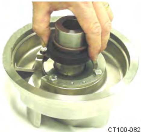
Figure 39 - Push Rotary Seal Down
