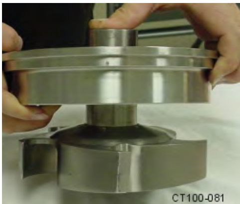
Figure 38 - Move Rotary Seal Up Shaft
