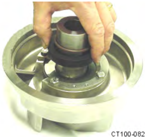
Figure 26 - Push Rotary Seal Down
