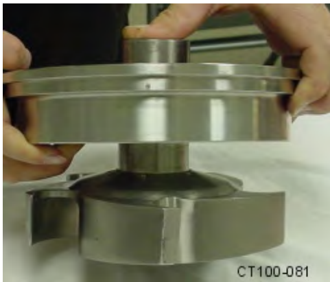
Figure 25 - Moving Rotary Seal Up the Shaft
