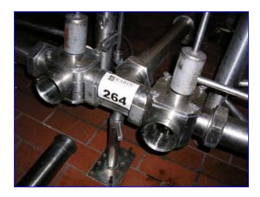
The Koltek Shutter Valve is a manually or pneumatically operated valve, designed for use in the food, chemical, pharmaceutical and other industries where sanitary designs are required Koltek valves meet 3A standards and are USDA approved for dairy, meat and poultry plants.
