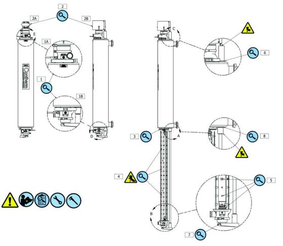
Figure 8-1A Recommended Inspection Points
