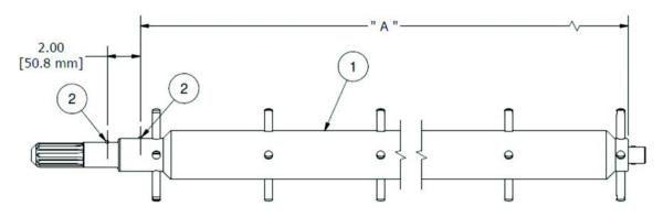
Figure 8-5. Seal Pin Locations for Rotors with Internal Bearings
