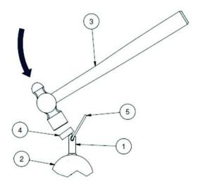
Figure 8-10. Repairing a Damaged Blade Pin 1. Blade pin 2. Rotor 3. Hammer
