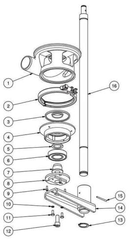
Figure 8-11. Lower Bearings. Non-Hold Down Style
