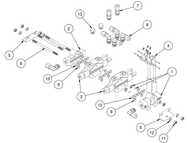
Figure 8-14. Stack Valve Assembly
