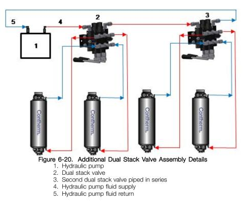
Figure 6-20. Additional Dual Stack Valve Assembly Details
