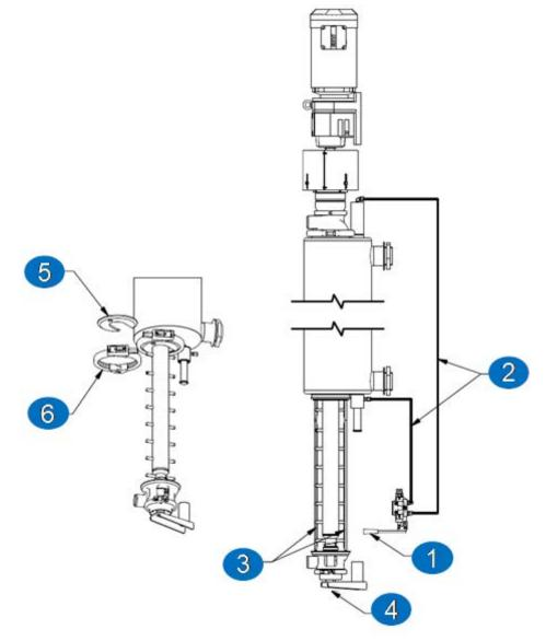
Figure 7-1. Hydraulic Rotor Lift System
