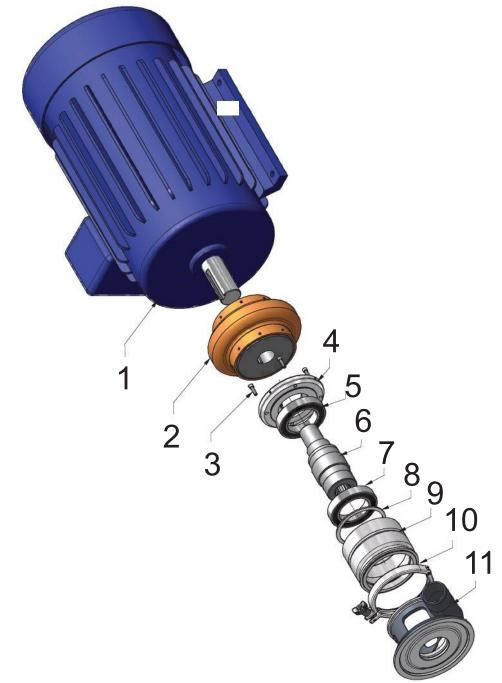
Figure 8-13. Upper Bearings, Direct Coupled, Electric Drive Motor
