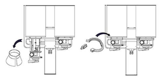
Figure 8-8C. Removing the Blade Funnel
