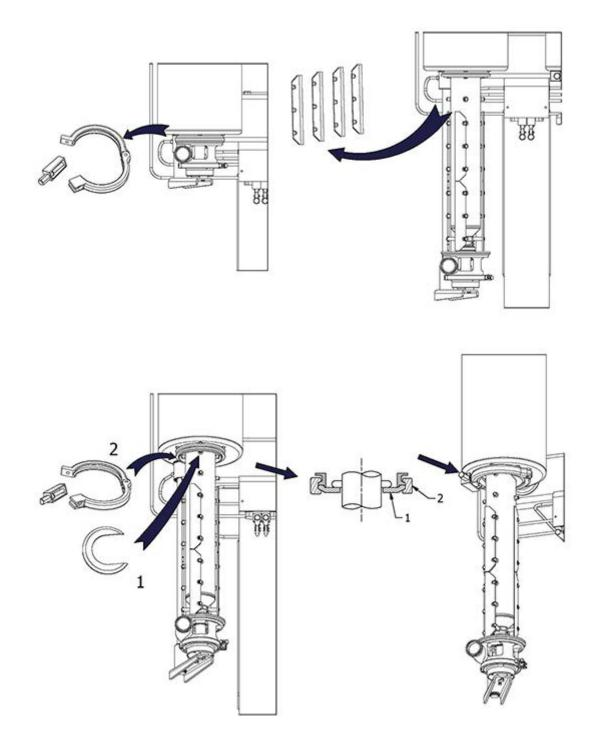
Figure 7-2A. Installing the Rotor Helper Plate
