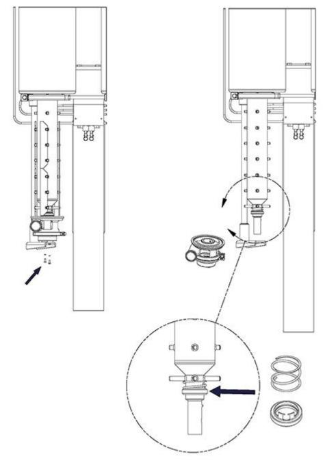
Figure 7-2B. Using Helper Plate to Access Lower Head & Seal Components
