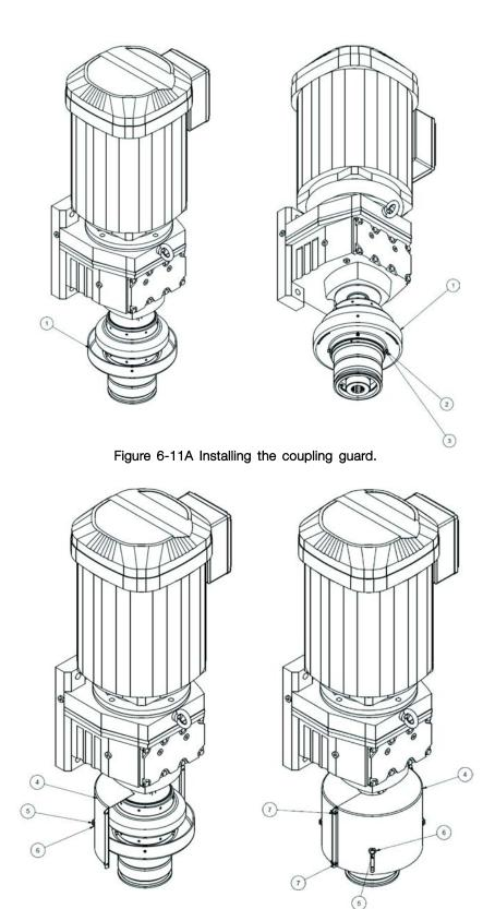
Figure 6-11B Installing the coupling guard continued
