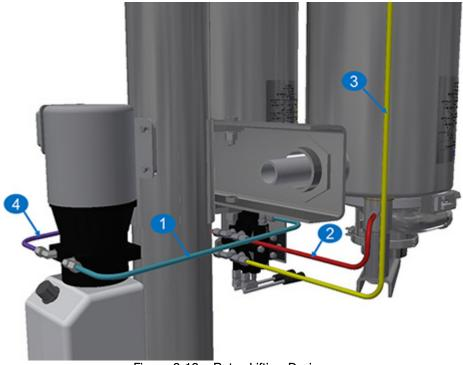
Figure 6-18. Rotor Lifting Device
