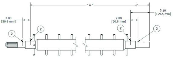
Figure 8-4. Seal Pin Locations for Rotors with External Lower Bearings
