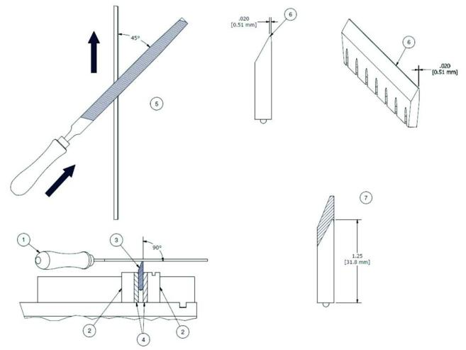
Figure 8-9. Dressing the Contherm™ Scraping Blades
