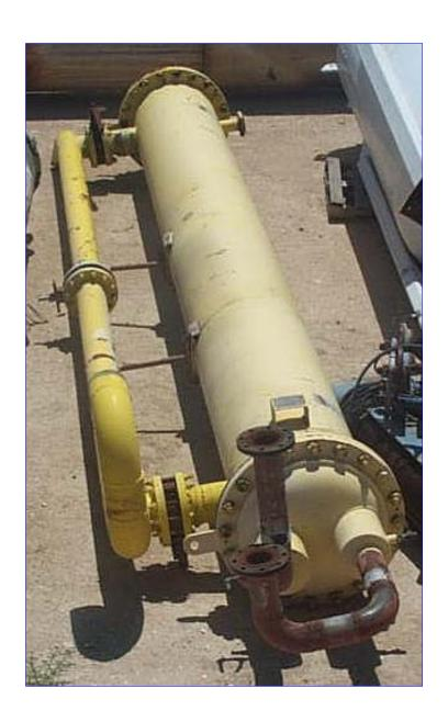
E.L. Nickell Tube-In Shell Heat Exchanger 1992, D – Superheater, max 100psi at 225F, minimum temperature -20F at 100F, 4in flange in-outlets, 24inD shell, 150 1 in carbon steel tubes, 2 pass, .5in drain, 25inDx21ftL
