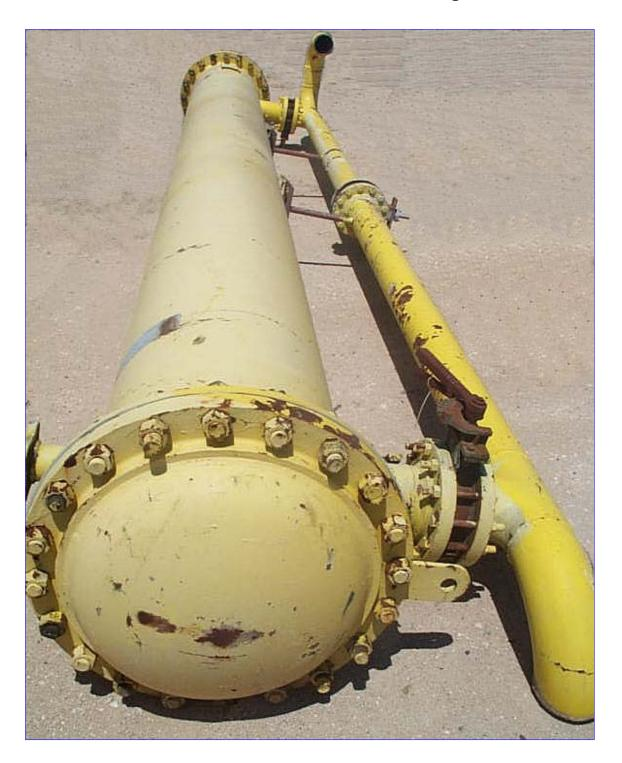
E.L. Nickell Tube-In Shell Heat Exchanger 1992, D – Superheater, max 100psi at 225F, minimum temperature -20F at 100F, 4in flange in-outlets, 24inD shell, 150 1 in carbon steel tubes, 2 pass, .5in drain, 25inDx21ftL
