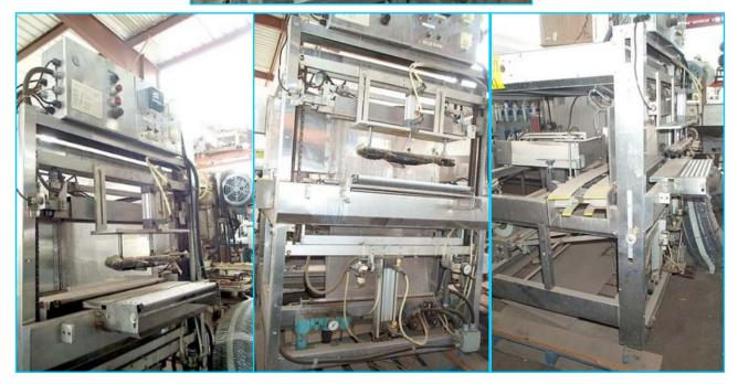
Great Lakes Corp. Heat Tunnel, Belt Stainless Steel 26 in. L, Heat Tunnel Box dimension 34 in. L, 35 in. W x 21 in. H. Sew Euro Drive-MFG, 0.7 hp, 460/230 volt, 3 phase, 1.5/3.0 amp, 60 Hz, 880 rpm, Output 72-362. Overall Dimensions 58 1/2 in. L x 38 in. W x 54 in. H.
