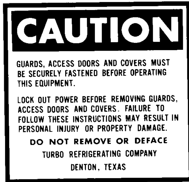
Figure 2-2 Warning Label on Access Panels
