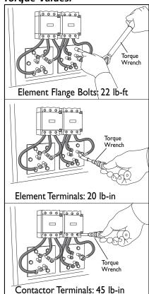
Power wiring shown in approximate factory-installed location
