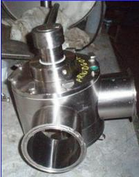
Working Principle: A polytetrafluoroethylene (PTFE) shutter is operated by means of a handle or an actuator. A spring washer system presses the shutter against the internal cylindrical surface of the valve body, ensuring a tight seal.
