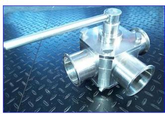
Working Principle: A polytetrafluoroethylene (PTFE) shutter is operated by means of a handle or an actuator. A spring washer system presses the shutter against the internal cylindrical surface of the valve body, ensuring a tight seal.
