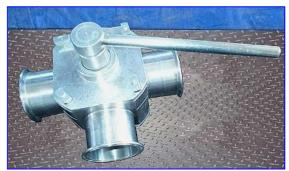
Working Principle: A polytetrafluoroethylene (PTFE) shutter is operated by means of a handle or an actuator. A spring washer system presses the shutter against the internal cylindrical surface of the valve body, ensuring a tight seal.
