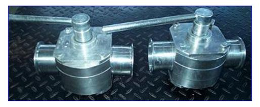
Working Principle: A polytetrafluoroethylene (PTFE) shutter is operated by means of a handle or an actuator. A spring washer system presses the shutter against the internal cylindrical surface of the valve body, ensuring a tight seal.
