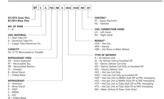
\* Copper and aluminum tube coils only.
