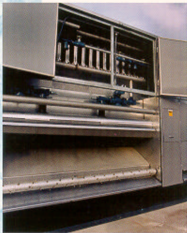
Breaker bar sizing mechanism gives operator control of ice size.
