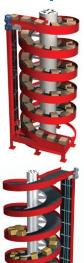
Central to our design is the Ryson proprietary slat-style belts designed with rolling friction without any sliding movements or wear strips. This facilitates a small footprint, high speed, low noise, low maintenance and a long life. Ryson Spirals are available in powder coated carbon steel, hybrid, stainless steel, washdown and freezer versions.
