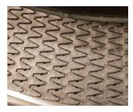
Nesting Slats: Nesting slats are used in the Mass Flow and Narrow Trak Spirals that convey small loads including loose bottles, cans, jars and similar containers. The conveying surface is flat without gaps, facilitating a smooth and reliable product side transfer. This can be done in a single file or in mass. They are available in 6", 9", 10", 16" and 20" wide slats.
