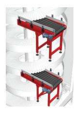
Loads can enter or exit the spiral in the up or down rotation. This is a perfect application for multi-level warehousing and order picking operations. This concept is also commonly used in applications where a single spiral connects multiple production or packaging elevations.
