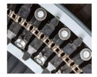
**Proprietary Slat Belt:** This innovative belt enables a low rolling friction operation without any sliding movements or wear strips. The belt is pulled by a heavy duty steel roller chain and the slats are supported by precision steel roller bearings which ride on a polyurethane surface. This arrangement effectively takes up the side forces created by a tight radius and at the same time increases the load
